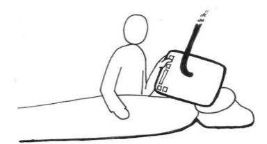
**Figure 1**: Concept of a projection display on a radiation shield directly controlled by the physician.
