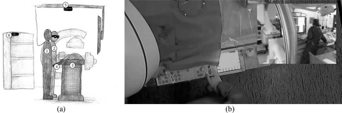
Fig. 1: (a) Sketch of the experimental setup in the intervention room: (1) technician, (2) neuroradiologist with eye tracking glasses, (3) patient table, (4) control panel of the angiography system, (5) top view camera, and (6) total camera. (b) Picture-in-picture presentation of top view camera and back view camera.
