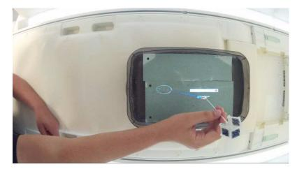
Figure 5: View of the projected scene from above with the wide-angle camera. Red is the insertion point, blue is the needle under the surface, and the faint green circle with the white contour is the target. The thickness and color of the virtual needle indicate depth.
