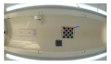
Figure 3: Estimation of the fixed ChArUco marker pose for registration of the MRI coordinate system with the camera coordinate system.
